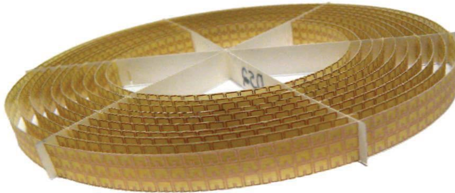
Figure 12. A microwave invisible cloak - might be useful for evading radar [64]. It is worthwhile to note here that radar detects the microwave sent from its antenna, after it is reflected back from a remote target.
